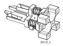
The actuator radius and the actuator incline is set through the position of the locking nuts
