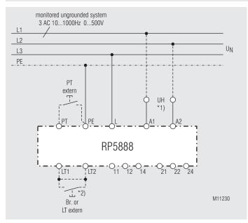
Monitoring of an ungrounded voltage system.
