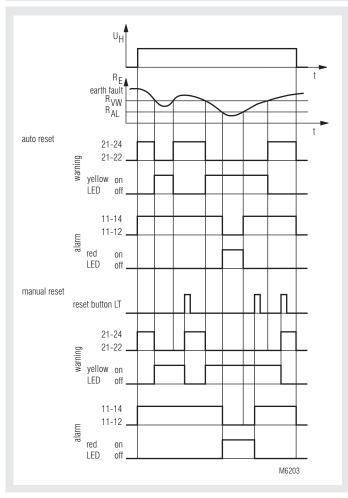
Function: de-energized on trip With function energized on trip, the status of the relay contacts 11, 12, 14 and 21, 22, 24 is inverted
