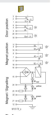
Fig. 2: Solenoid locking deactivated: Magnet released, actuator and key inserted, Door closed
