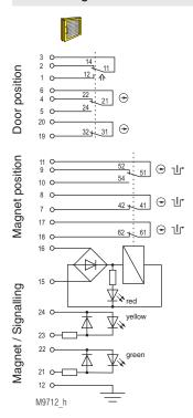
Fig. 1: Solenoid locking activated: Magnet locked, actuator and key inserted, Door closed
