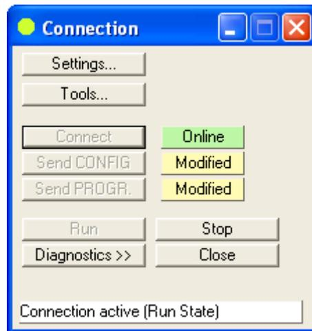
**Send CONFIG:** Transmits the configuration to the SMX100 module.
