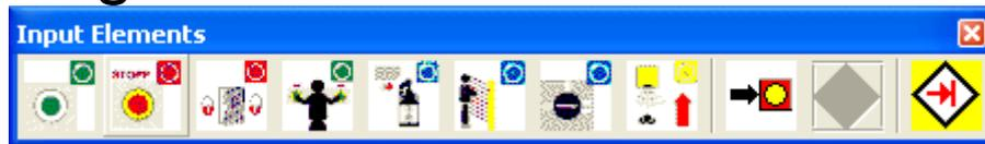
The input elements deliver the data about operating status of the plant monitored by the SMX100- module. These components, which, from the point of view of the SMX100- module, are outside the device, can only be inserted and configured in the terminal plan.
