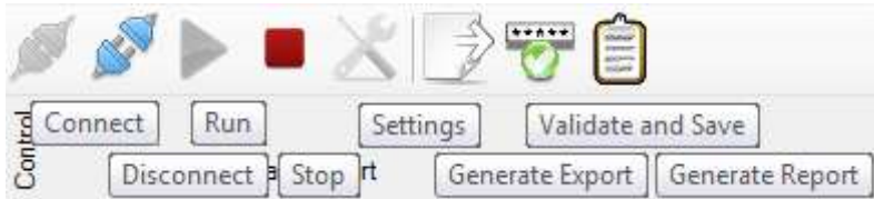
Fig. 29: Icon tools in the Device Interface – disconnected
