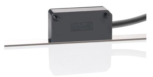
The series IMAX is a pseudo-absolute magnetic length measuring system. Pseudo-absolute means, that the absolute code is recognized through a one-time movement after power up. At this point the IMAX measures really absolute. So it's possible to have a measuring length up to 1000 meter with an absolute encoder resp. sensor of only 50 mm length.
