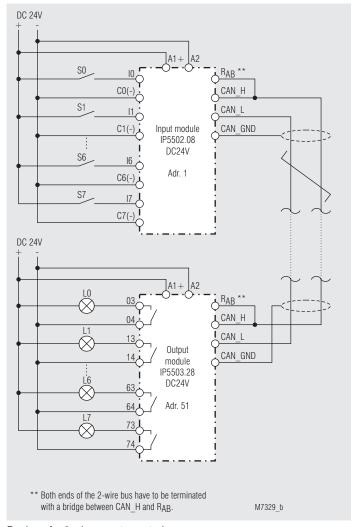
Design of a 2-wire remote control Switch position: Plug & Play
