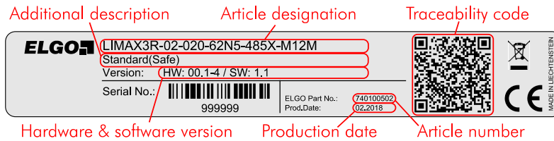
Fig. 2: Type label for identification of the sensor
