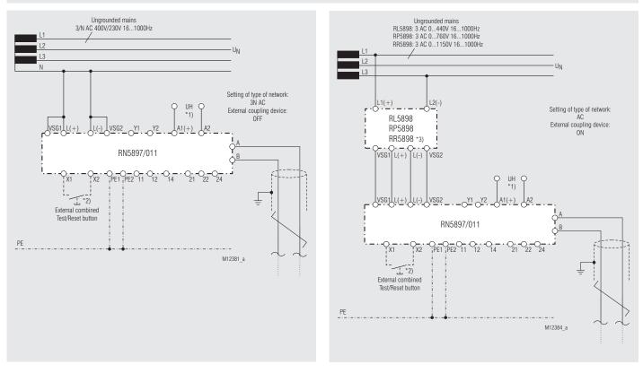
\*1) Auxiliary voltage U<sub>H</sub> (A1(+)/A2) can also be sourced from the monitored voltage system. The voltage range of the auxiliary supply has to be taken into account.
