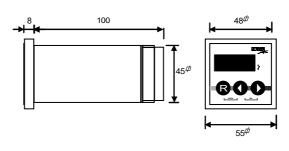
48 mm without front frame 55 mm with front frame
