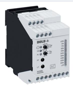
The insulation monitors MK 5880N and MH 5880 of the VARIMETER IMD family provides best insulation monitoring of pure three-phase and AC IT systems in a state of the art way fulfilling the relevant standards. The adjustment of the setting values is simple and user friendly done on 2 rotary switches on the front of the device. The MH 5880 also has a galvanic separated analogue output and a 11 step LED chain for display the actual insulation value.
